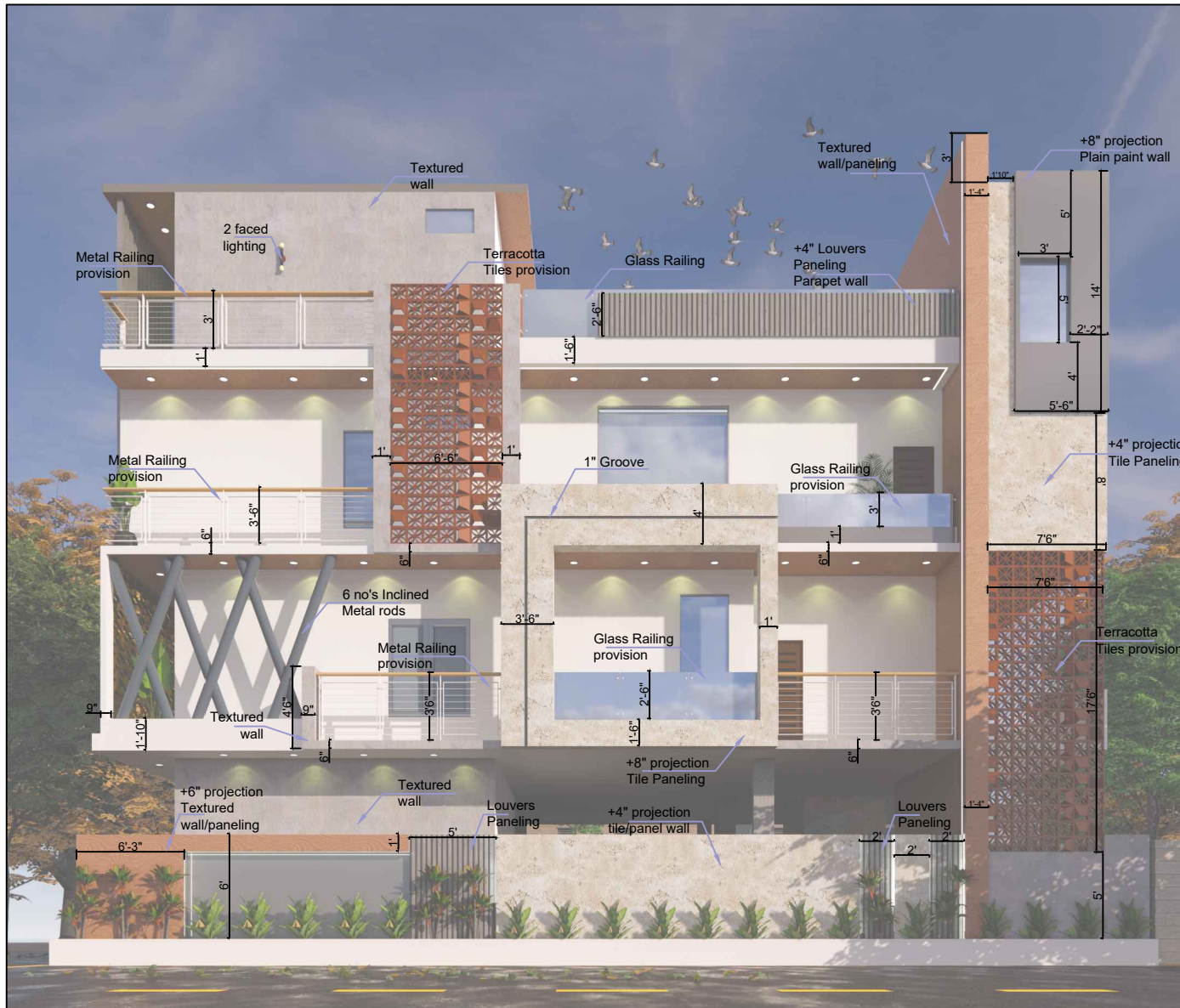
DETAILED ELEVATION @South View
