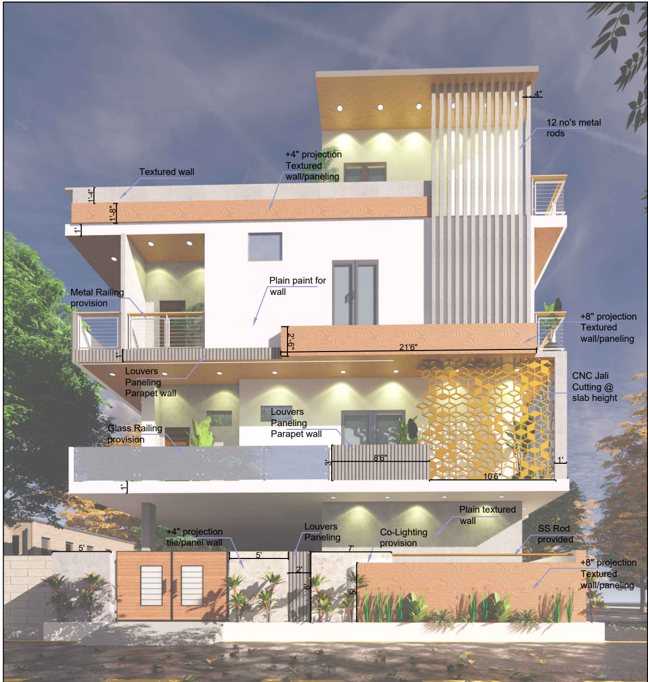
DETAILED ELEVATION @West View
